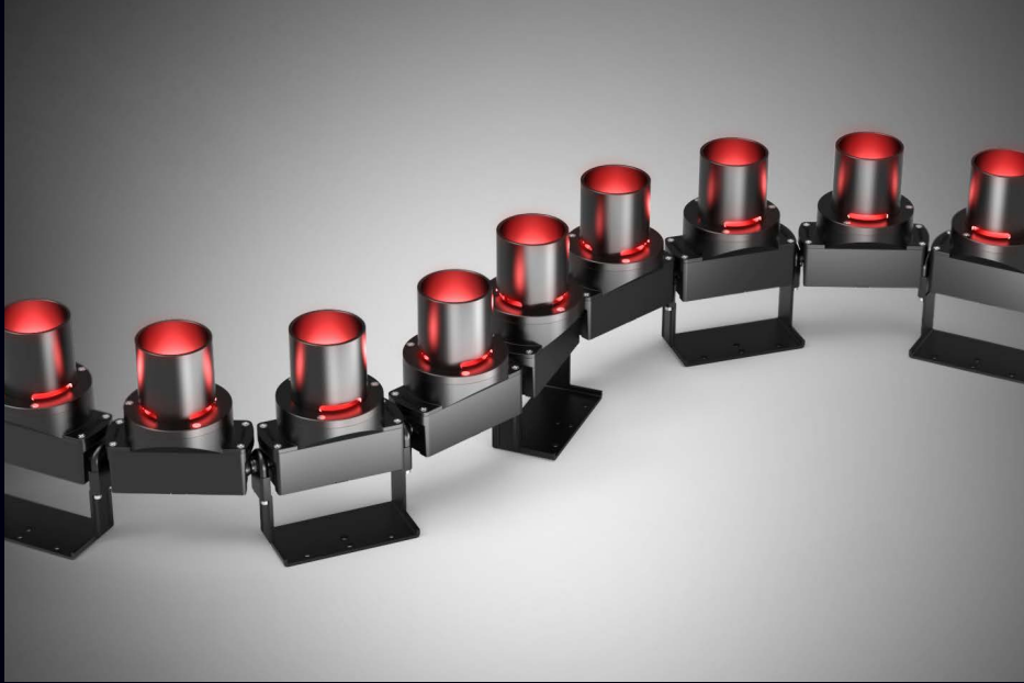
3D LED Flex 40 IP66 system. Each module comprises 4 x Luxeon Z red LEDs with a Gaggione ultra-narrow beam lens, and custom height anti-glare snoot. Each module is individually addressable via DMX
