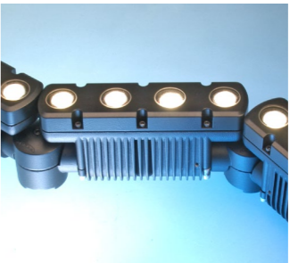
Serpentine with UV stop glass windows 4 x 3.5W Citizen or Sharp COB LEDs with reflectors
